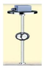
A Simple construction of float and guide pipe made up Non magnetic materials . Magnetic Float Moved\s with Level Over guide Pipe, So that the resistance of the PCB inside the pipe change which is converts into 4-20Ma / 0 to 5 V output.
